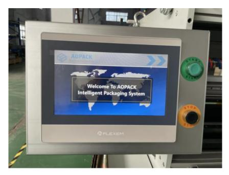
All settings can be entered directly from a large touching screen panel within one minute. Additionally, with the different sizes of screen, their memory capacity are also affected. Interactive touch screen control panel with 10" diagonal, START & STOP button.
